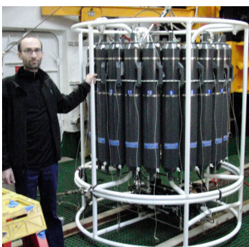
Figure 2: Pierre St-Laurent, CCPO, with a CTD Rosette. The CTD is attached to a frame fitted with a number of large water-collecting bottles called Niskins. The instrument together with the bottles is called the CTD Rosette.
