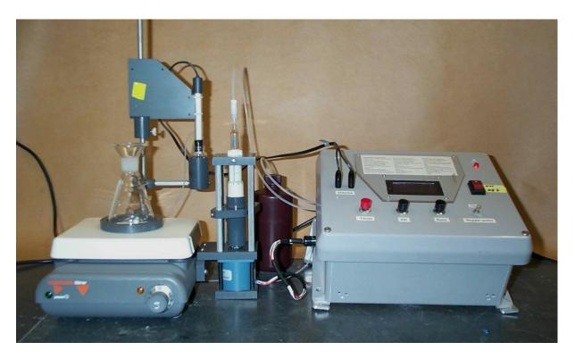
A computer may be connected to the back of the electronics box via an RS232 port in order to communicate with the titrator and to download data. The computer connection is required to capture the titration data to disk. A Windows program called Txtools4.14 has been provided for
