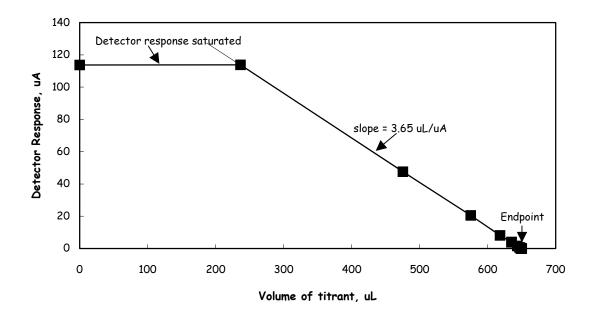
Calculate the reciprocal of the slope of the linear portion of the titration curve by dividing the change in volume of titrant by the change in detector current. The slope will depend on the concentration of the thiosulfate and the volume of the bottle. The titrator controller uses the slope to determine how much titrant to add. Each time the titrator prepares to make an addition it makes the following computation:
