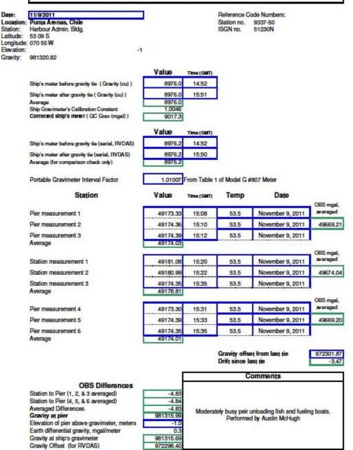
Note about Elevation of Pier: If pier is below the ship's gravimeter, this value is negative. If above, positive.
