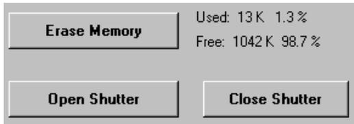
**Erase Memory:** Allows you to erase data stored within the instrument. Each data measurement taken by the meter uses approximately 20 bytes of memory: the total memory capacity is approximately 50,000 measurements. Not applicable for RT meters.
