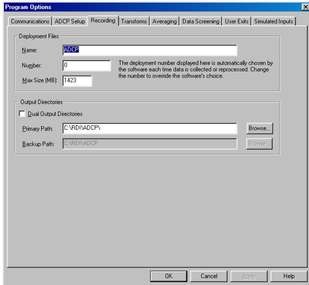
**Figure 8. Recording Tab**
