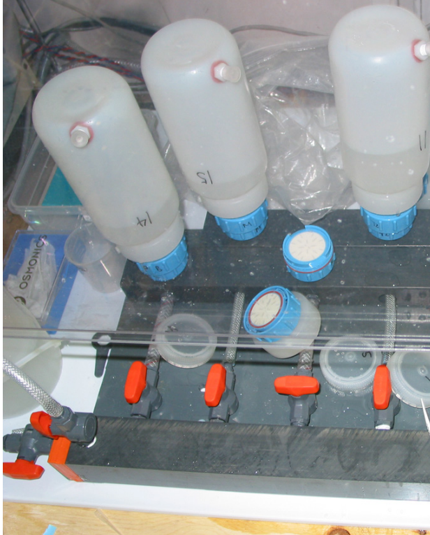
Figure 3. An example of a 1 L offline filtration method as used routinely on CLIVAR A16N, A16S, VERTIGO, and GEOTRACES IC expeditions. Pre-cleaned 1L LDPE bottles are modified with closing air vents at bottom. Sample is quickly transferred from the GO-FLO into the 1 L LDPE bottle which is then capped conventionally. Once returned to a Laminar Flow bench environment, the top is substituted for a tapered adaptor which has a mated 47 mm MFS filter holder with preloaded 0.45 \mu m Supor filter. The upstream orifice of the filter holder has been drilled out to twice standard diameter to minimize air-lock effects. Once samples are filtered under 25 to 40 mm Hg vacuum, they are transferred directly to sample bottles for further processing. Primary sample bottles and filter holders are reused after TM-clean DI water rinsing. More information available from J. Bishop ( jbishop@berkeley.edu ) or Todd Wood ( tjwood@lbl.gov ).
