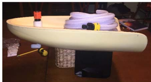
Surface sampler: modified otter boat, also known as “Big Jon”
