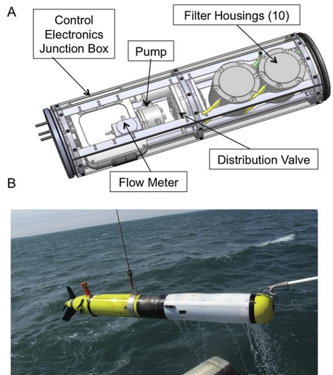
Fig. 1. (A) Schematic of SUPR components installed on REMUS 600. (B). SUPR-REMUS being recovered from the research vessel R/V Tioga.
